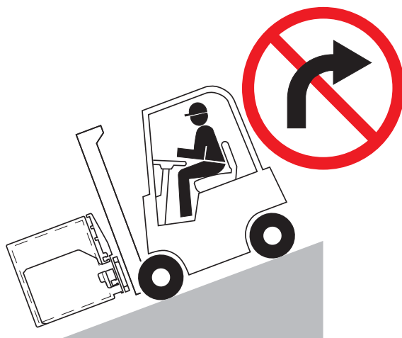
禁止坡上转弯 No turning on ramp
