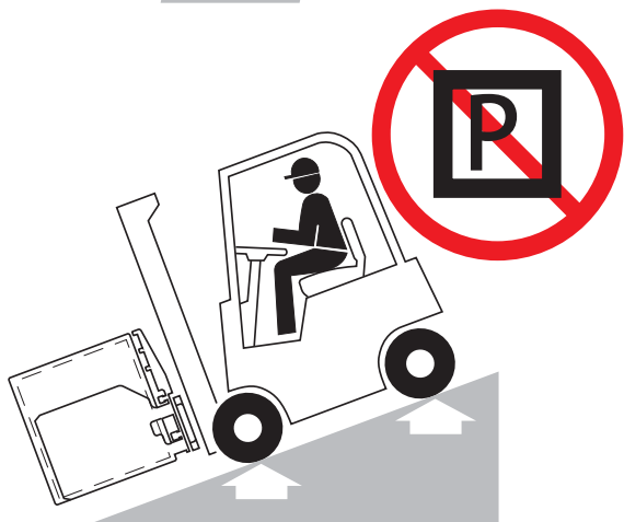
禁止坡上停车 No parking on ramp
