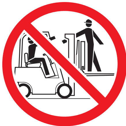
禁止穿越门架 No reaching through mast
